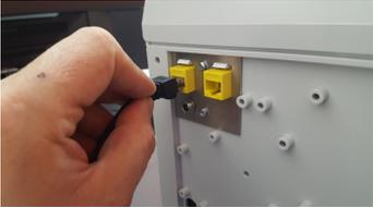
Optionally plug in the network cable of the MFP in the box, It will be patched trough to the network outlet.
