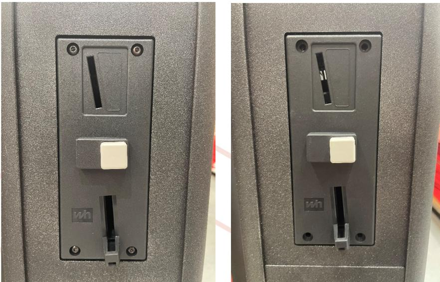
9. Pull the coin acceptor front and wiggle it loose. If this does not loosen the coin acceptor, pull off the top and push the coin acceptor out from within with your hand.
