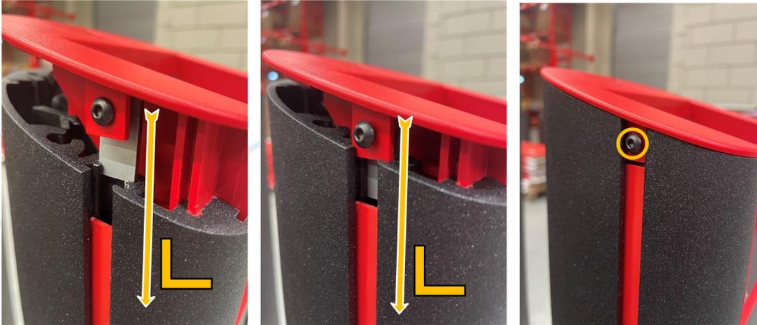
15. Screw it down until it is just tightened with the H2 Allan key.
